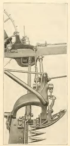
A wide hinge coupling is a great advantage as it gives this cutter-bar great steadiness. The cutter-bar is connected to the hinge coupling by means of two heavy removable steel pins
