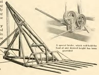
Lifting Arms are Strengthened: The Deering swinging hay stacker has a rectangular base. The lifting arms are attached to the turning mast and are strengthened by truss rods which prevent the pitcher head from twisting out of position when the load is improperly and unevenly distributed. After the pitcher head has been raised, it can be locked and the hay dumped in the middle or at either
