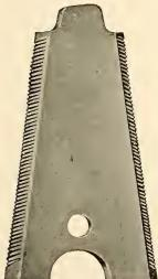
The ledger plate has serrated cutting edges
