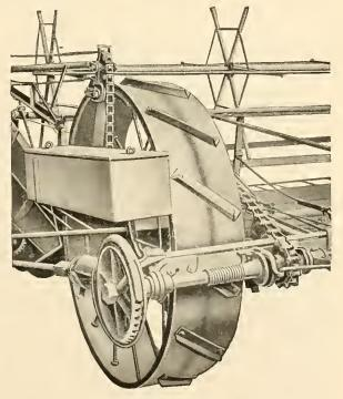
Main wheel and main gear on header-binder
