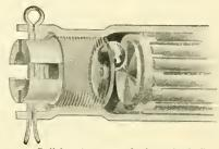
Main gear shaft and crank shaft with frictionless ball and roller bearings
