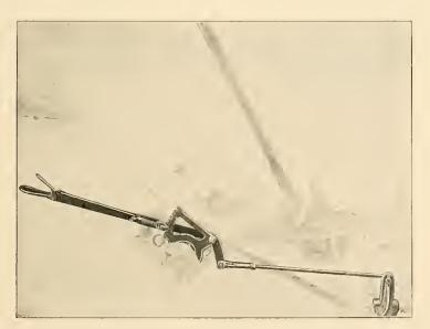
Showing tilting lever, quadrant and connections
