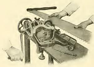
Gumming a cross-cut saw
