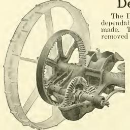
Note compact construction of internal and bevel gears
