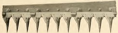
Section of New Ideal mower cutter-bar
