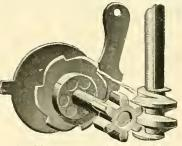
Steel twine-holding disk and pinion
