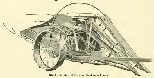
The Deering Corn Binder Saves Labor and Expense: The Deering Ideal corn binder cuts the standing corn, binds and discharges it as fast as the horses walk. Like the grain binder, it makes a big saving possible, not only in manual labor, but also in the number of hands required and wages and board for extra men. At the same time, the corn binder does from five to eight times as much work per day under average conditions as a man would do. Tall and short corn is handled with equal ease.
