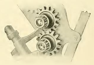
Elevator bearings partly exposed to show rollers
