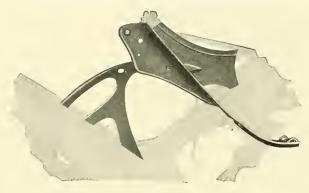
Shape of needle and breastplate forces the straw away from the breastplate, preventing clogging at this point
